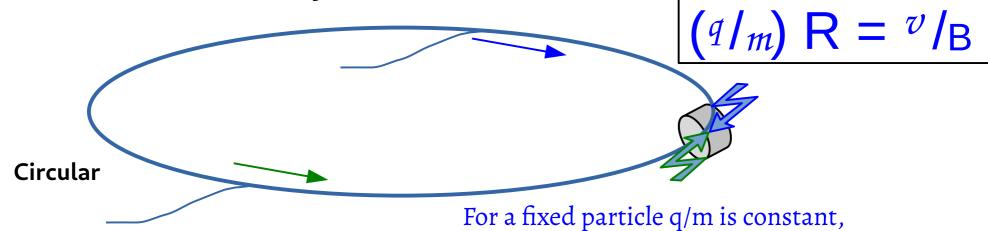
So magnetic field B must increase with velocity v.
