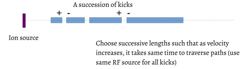
eg. Stanford Linear Accelerator, 3.2km long, accelerating ele to 50 GeV
