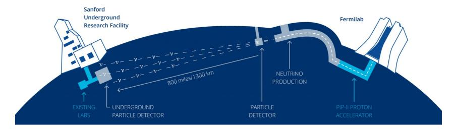
Consider the DUNE experiment (Deep Underground Neutrino Experiment) 70k tons of Liquid-Argon
