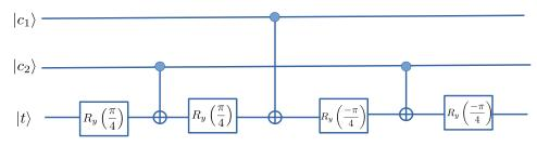
This circuit takes  $|c_1, c_2, t\rangle$  to  $e^{i\theta(c_1, c_2, t)}|c_1, c_2, t \oplus c_1c_2\rangle$ . Determine the phase  $\theta(c_1, c_2, t)$ . (8)
