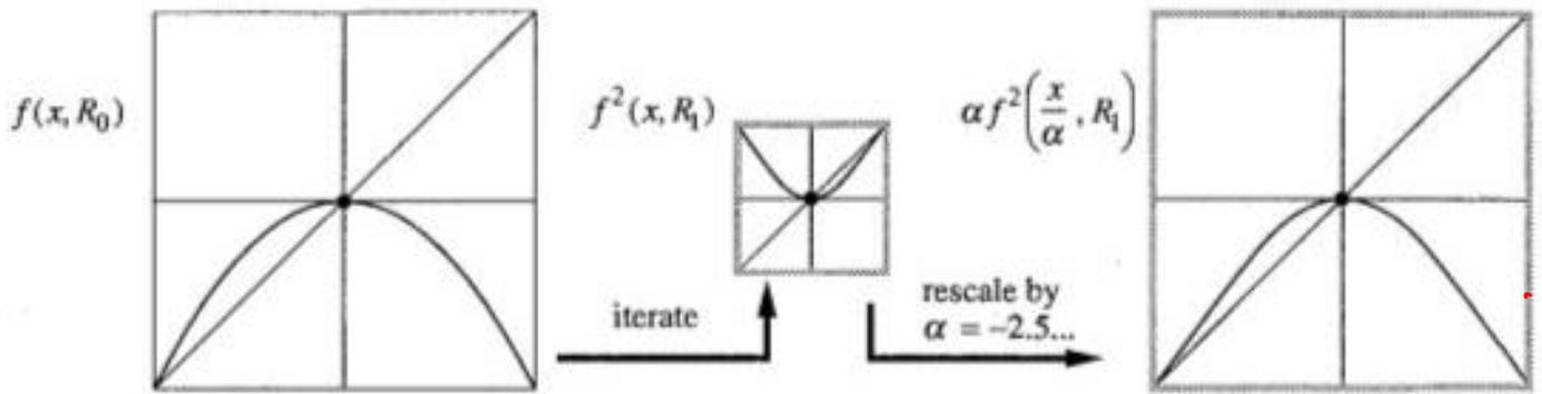
Take the middle figure. Blow it up by a factor  $|\alpha| > 1$  in both the directions. Also let  $(x, y) \rightarrow (-x, -y)$ .
