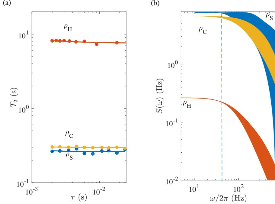
**Figure 3.6:** (a) The experimental decay constants (dots) of  $^{13}\text{C}$ -Chloroform at various  $\tau$  delays for single spin states  $\rho_H = I_x$ ,  $\rho_C = S_x$ , and the singlet state  $\rho_S$  at 500 MHz. The solid lines correspond to decay constants obtained from the best fit by the 3-Lorentzian model as described in Eq. 3.13. (b) The corresponding noise spectra.
