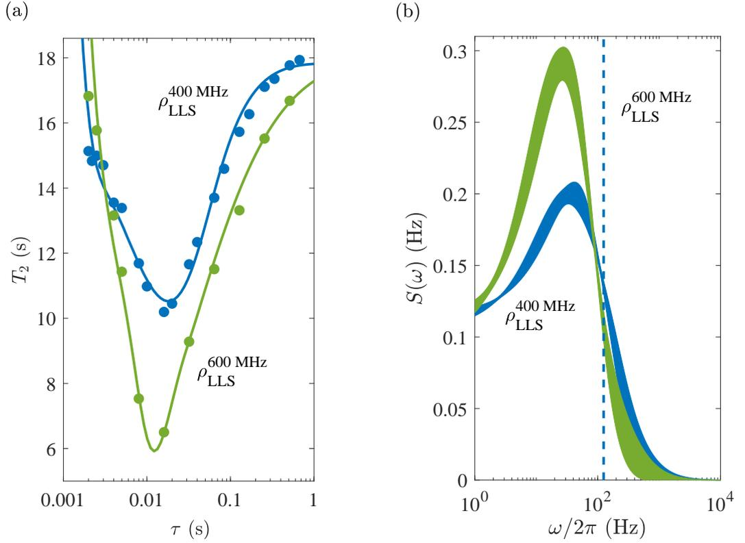
**Figure 3.4:** (a) The experimental decay constants (dots) at various  $\tau$  delays for the singlet state  $\rho_{\text{LLS}}$  at two different magnetic fields, i.e., 400 MHz and 600 MHz as indicated. The solid lines correspond to decay constants obtained from the best fit by the 3-Lorentzian model as described in Eq. 3.13. (b) The corresponding noise spectra.
