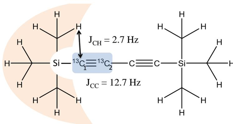
**Figure 2.2:** Structure of 1, 4-Bis (trimethylsilyl) butadiyne. Here protons in the shaded area act as ancillary spins which provide polarization to  $^{13}\text{C}$ - $^{13}\text{C}$  singlet-order.
