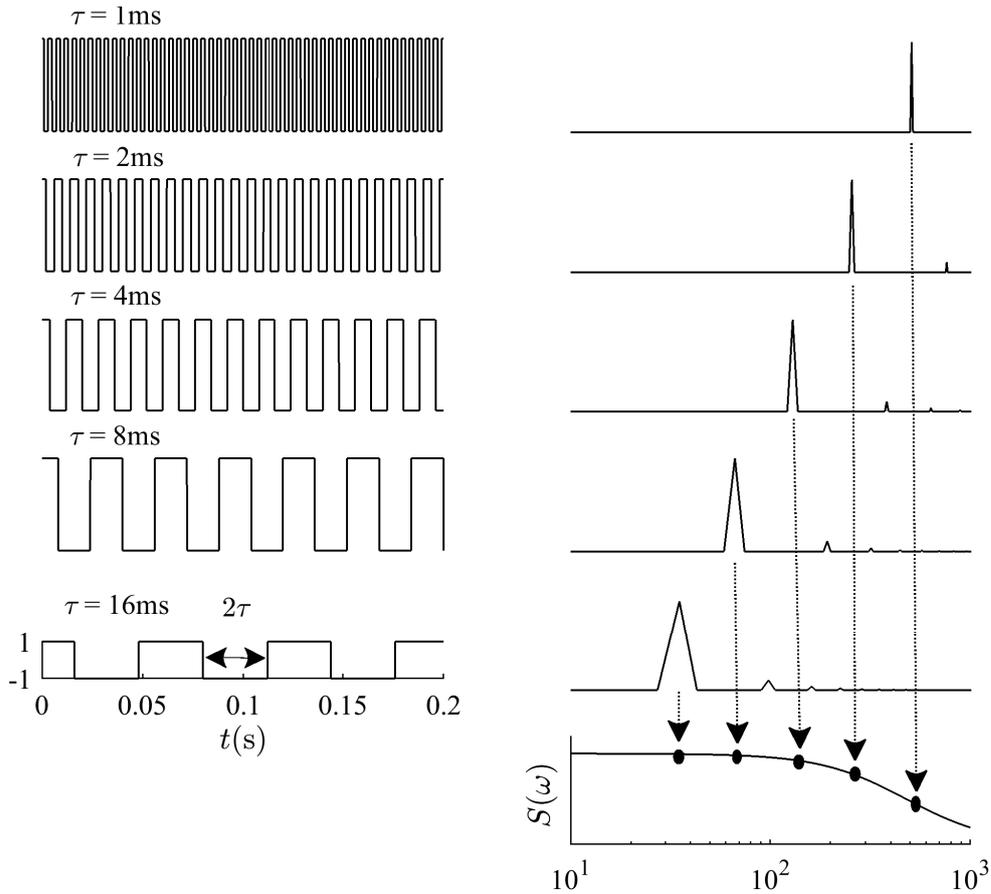
**Figure 3.1:** The modulation functions  $f(t, T)$  (left column) and the corresponding Fourier transforms, i.e., Filter functions  $F(\omega, T)$  (right column). The 1st order sampling points of the filter functions are illustrated using a schematic spectral density function  $S(\omega)$  as shown in the lowest trace of the right column.
