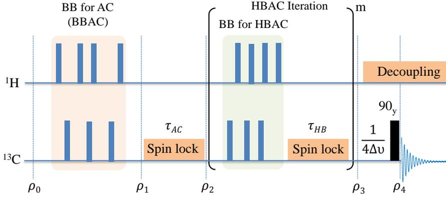
**Figure 2.3:** Pulse sequence for the preparation and enhancement of  $^{13}\text{C}$ - $^{13}\text{C}$  singlet-order using  $^1\text{H}$  spins. Here  $m$  can take integral values 0, 1, 2,  $\dots$  etc.
