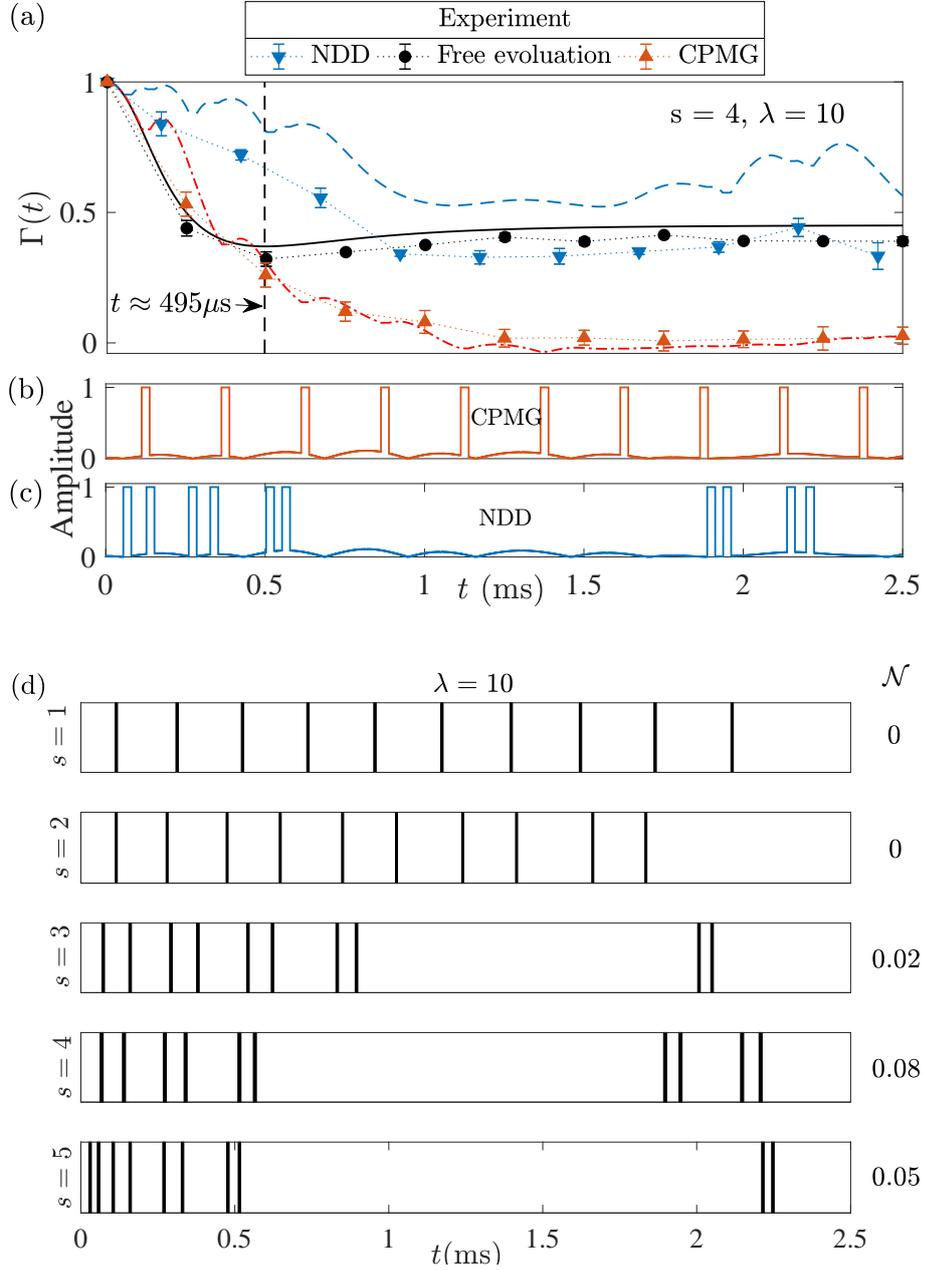
**Figure 4.4:** (a) Theoretical and experimental (symbols) decoherence functions with free-evolution (smooth), CPMG (dash-dot) (b), or NDD (dash) (c) sequences. In (b) and (c) one particular noise realization is interleaved with  $\pi$  pulses. (d) Optimal DD sequences for various ohmicity parameter  $s \in \{1, 5\}$ . Corresponding values of non-Markovianity measure are also indicated.
