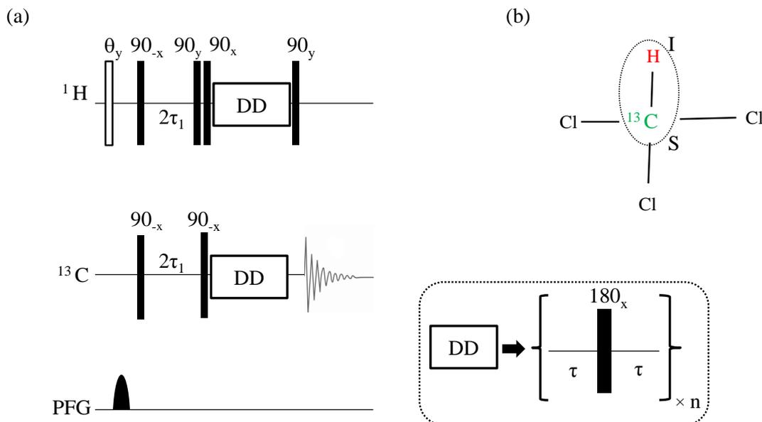
**Figure 3.5:** (a) Pulse sequence to measure noise spectrum in a heteronuclear spin system. (b) Molecular structure of Chloroform. Here singlet state is prepared on  $^1\text{H}$  and  $^{13}\text{C}$  spins with a coupling constant  $J_{\text{CH}} = 209$  Hz between them. The CPMG DD sequence is shown in the inset.
