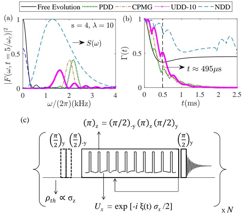
**Figure 4.3:** Noise spectrum (dashed line) for BLP non-Markovian environment corresponding to  $s = 4$ ,  $\lambda = 10$  and filter-functions  $|F(\omega, t)|^2$  at  $t = 5 \omega_c^{-1}$  for various DD sequences as well as for free-evolution (a) and corresponding decoherence functions (b). (c) Circuit used to apply dynamical decoupling along with noise modulation.
