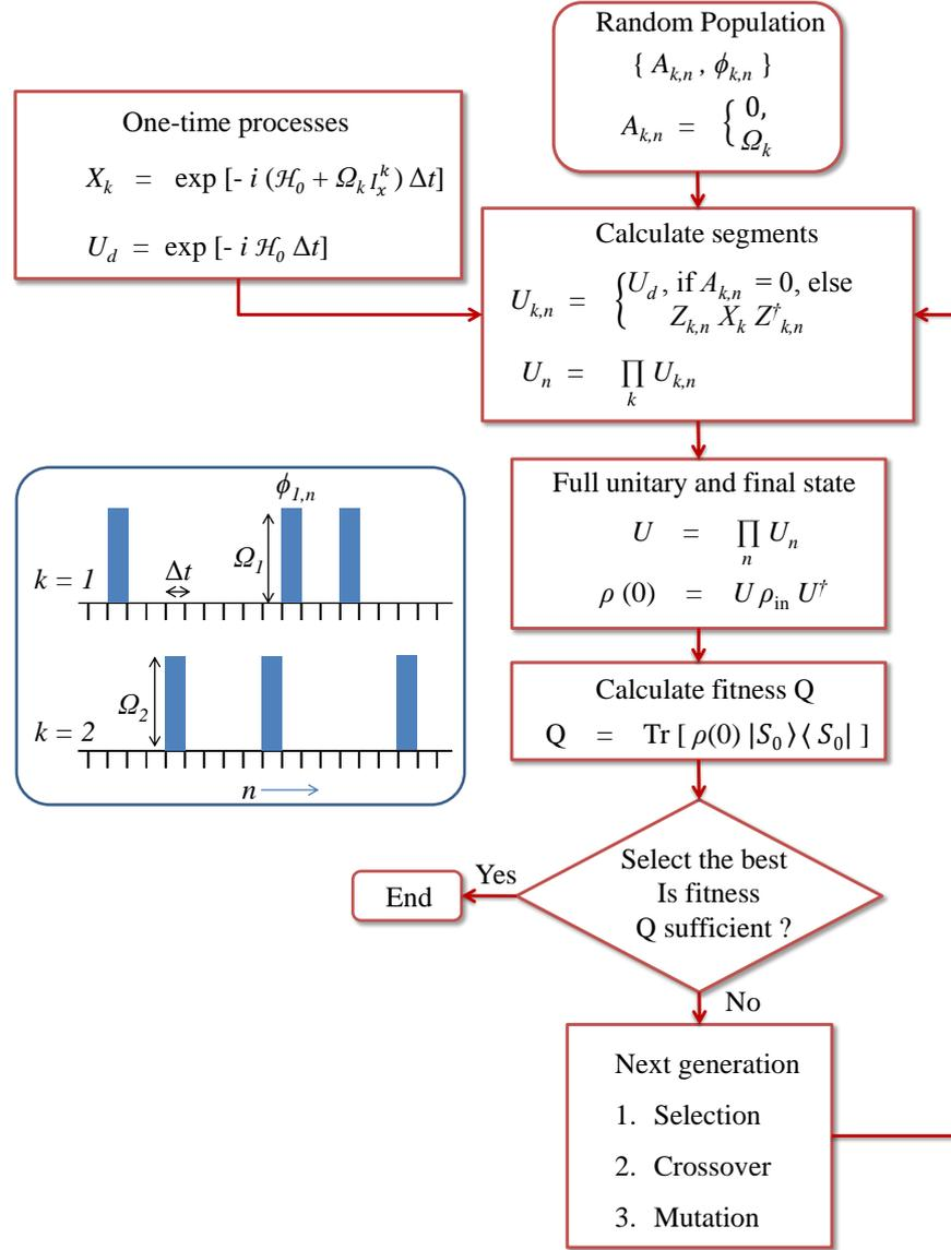
**Figure 2.1:** The flowchart describing BB optimal control with genetic algorithm. A schematic diagram of BB control is shown in the inset, wherein each rectangular box corresponds to a full power RF pulse, called a *bang*.
