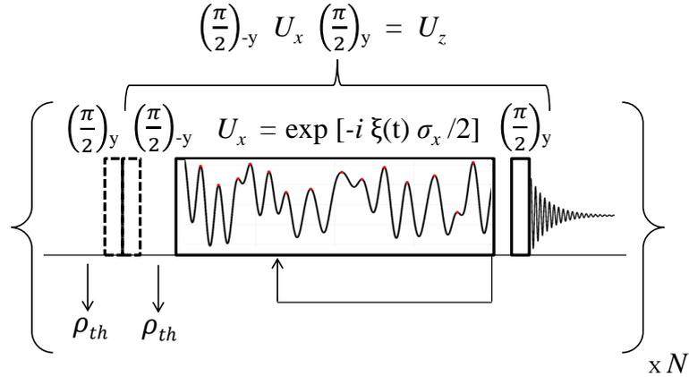
**Figure 4.1:** NMR pulse-sequence used to implement a non-Markovian dephasing dynamics. Here  $\rho_{th} = (\mathbb{I} + \epsilon\sigma_z)/2$  is the initial thermal state with purity factor  $\epsilon$ . The final signal is obtained by averaging over  $N$  independent realizations of the stochastic process  $\xi(t)$  as in Eq. 4.4.
