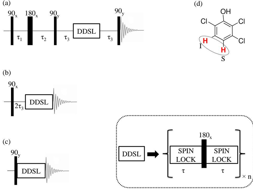
**Figure 3.2:** Pulse sequences used to measure the noise spectrum of (a)  $\rho_{\text{LLS}}$ , (b)  $\rho_{\text{LLC}}$ , and (c)  $\rho_{\text{SL}}$ . Here  $\tau_1 = 1/(4J)$ ,  $\tau_2 = 1/(4J) + 1/(2\Delta\nu)$ ,  $\tau_3 = 1/(4\Delta\nu)$ , and  $n$  is the number of times the loop is repeated. (d) Structure of 2,3,6-trichlorophenol. The CPMG DD sequence with spin-lock along  $x$ -axis is shown in the inset (DDSL).
