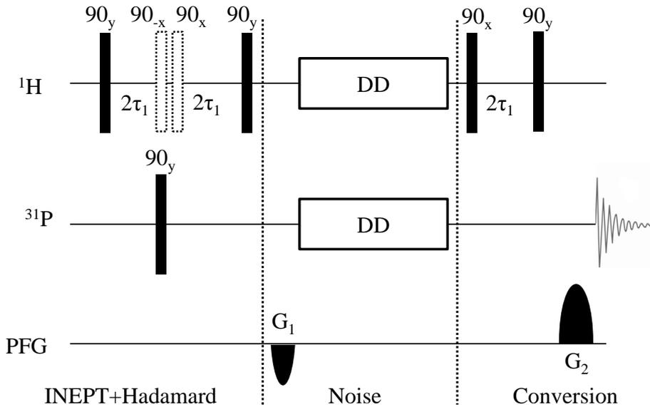
**Figure 3.7:** Pulse sequence to measure noise spectra of the MSSM states. An initial INEPT (insensitive nuclei enhanced by polarization transfer) [36] operation is used to transfer magnetization from  $^1\text{H}$  to  $^{31}\text{P}$ . The PFGs  $G_1$  and  $G_2$  are chosen such that  $\phi_2(k) = -\phi_1(k)$  to select out an MSSM state with a particular lopsidedness  $l(k)$ . A CPMG-DD sequence with composite  $\pi$ -pulses was used.
