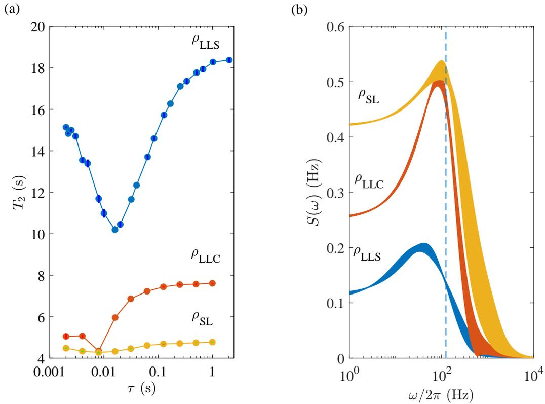
**Figure 3.3:** (a) Experimental decay constants (dots) of 2,3,6-trichlorophenol (averaged for both protons) in 400 MHz spectrometer for a range of  $\tau$  values and for different states as indicated. The solid lines correspond to decay constants obtained from the best fit by the 3-Lorentzian model as described in Eq. 3.13. (b) The corresponding noise spectral density bands. The dashed line at 125 Hz corresponds to the maximum harmonics sampled with  $\tau = 2$  ms.
