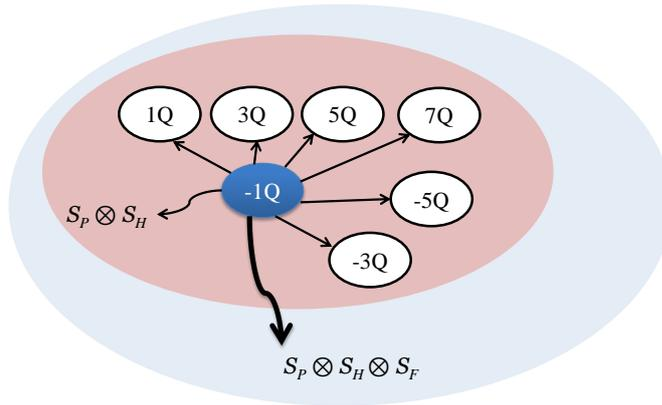
**Figure 5.3:** Leakage of information localized in MQC subspace corresponding to  $q = -1$ , i.e.  $\rho_{-1}^x(0)$ . Here  $S_P$ ,  $S_H$  and  $S_F$  represent Hilbert spaces corresponding to  $^{31}\text{P}$ ,  $^1\text{H}$  and  $^{19}\text{F}$  spins respectively. Quantitative analysis is shown in Fig. 5.4.
