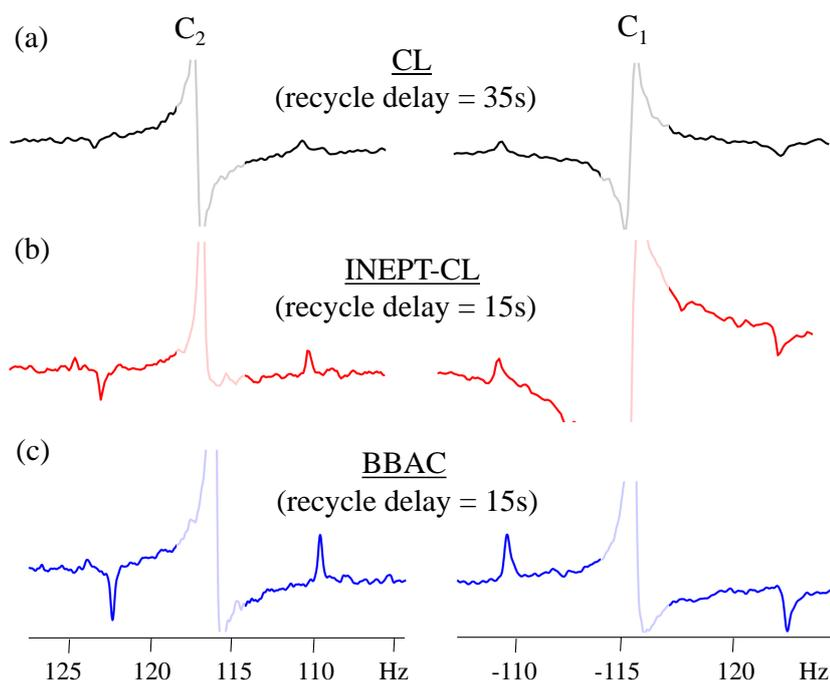
**Figure 2.5:**  $^{13}\text{C}$  spectra of BTMSB obtained by converting  $^{13}\text{C}$ - $^{13}\text{C}$  singlet-order at natural abundance into single-quantum coherence using: (a) only CL, (b) INEPT-CL, and (c) BBAC singlet sequences. All spectra were recorded with WALTZ-16 spin-lock (1.5 kHz,  $\tau_{\text{AC}} = 10$  s). The central peaks corresponding to  $^{13}\text{C}$ - $^{12}\text{C}$  pairs are de-emphasized.
