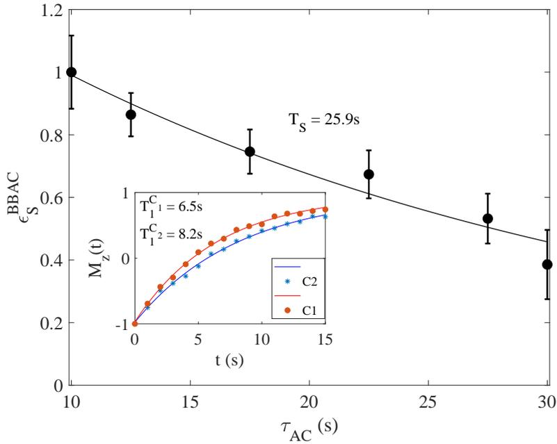
**Figure 2.7:** The decay of singlet-order versus spin-lock duration  $\tau_{\text{AC}}$ . The vertical axis is normalized w.r.t. the first data point. Inversion-recovery curves and corresponding  $T_1$  values of both carbons are shown in the inset.
