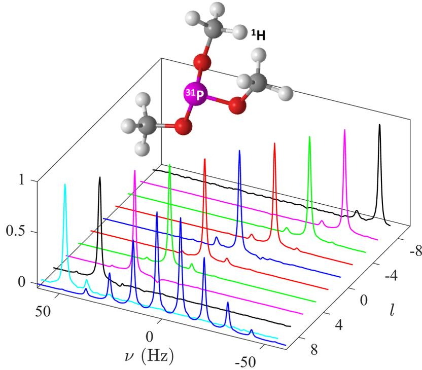
**Figure 3.8:** The spectral lines corresponding to various MSSM states with varying lopsidedness  $l$ . Each spectral line is individually normalized. The reference spectrum with all the lines is shown at the front. The structure of Trimethylphosphite is also shown at the top-left corner.
