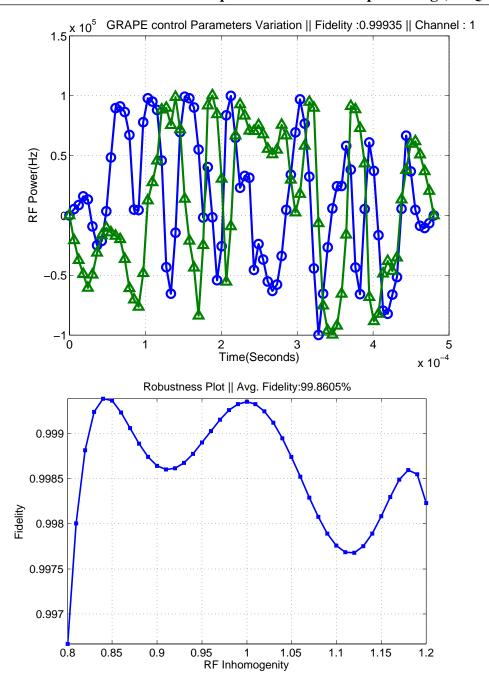
**Figure 1.6:** GRAPE generated RF profiles of  $\pi_x$  pulse on <sup>19</sup>F spins of iodotrifluoroethylene: X- component is shown in blue, Y- component is shown in green (top), and robustness profile against RFI (bottom).
