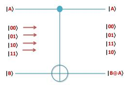
**Figure 1.2:** Circuit for the C-NOT gate.
