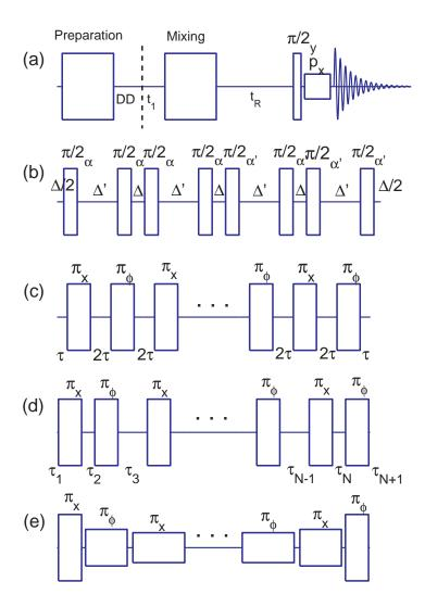
**Figure 6.1:** The experimental scheme (a) for studying the performance of DD on large spin-clusters and the 8-pulse sequence (b) implementing  $\mathcal{H}_1(\alpha)$ . In (b),  $\Delta' = 2\Delta + \tau_{\pi/2}$ , where  $\tau_{\pi/2}$  is the duration of each  $\pi/2$  pulse. The DD schemes are described in (c-e). The phase  $\phi$  is set to x for CPMG, UDD, and RUDD schemes, while it is alternated between x and -x for CPMGp, UDDp, and RUDDp.
