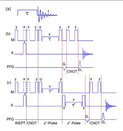
**Figure 5.4:** (a) Pulse sequence for single-quantum Torrey oscillation, (b) pulse sequence for NOON Torrey oscillation, and the RFI, (c) pulse sequence for measuring RFI correlation between  $^{1}$ H and  $^{31}$ P channels. In (b) and (c) except the variable duration ( $\tau$ ) pulses, all other pulses are  $90^{\circ}$
