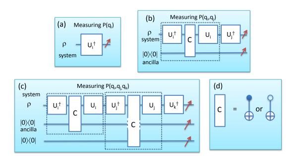
**Figure 4.2:** Circuits for measuring SEP (a), and two-time JP (b), and three-time JP (c). The grouped gates represent measurement in  $\{\Pi_0^t, \Pi_1^t\}$  basis. The operation C can be either CNOT gate or anti-CNOT gate, as described in the text. In (c) the second CNOT gate is applied between first and third spin. The pointer at the end in each circuit represents the measurement of diagonal elements of the density matrix. (d) Block C represents either CNOT or anti-CNOT gate.
