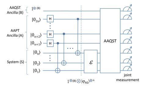
**Figure 3.2:** Quantum circuit for SSPT. Building blocks of the circuit involves initialization of the system and ancilla registers, encoding of the input states into subspaces of system-ancilla register, application of process  $\varepsilon$ , and finally AAQST.
