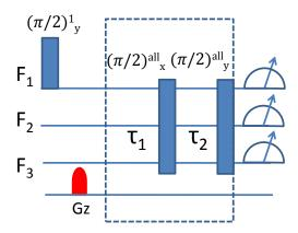
**Figure 2.3:** The pulse sequence for two qubit AAQST. A  $\frac{\pi}{2}$  pulse followed by a gradient prepares first spin into maximally mixed state. The pulse sequence corresponding to unitary  $U_1$  is shown inside the dotted block. Unitaries  $U_{int}(\tau_1)$  and  $U_{int}(\tau_2)$  are realized by delays  $\tau_1$  and  $\tau_2$ . The  $\frac{\pi}{2}$  are shown by solid boxes.
