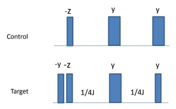
**Figure 1.5:** NMR pulse sequence for the C-NOT gate. Thin pulses are  $\frac{\pi}{2}$  pulses and broad pulses are  $\pi$  pulses. Delay  $\frac{1}{4J}$  represent free evolution under secular part of indirect spin-spin interaction.
