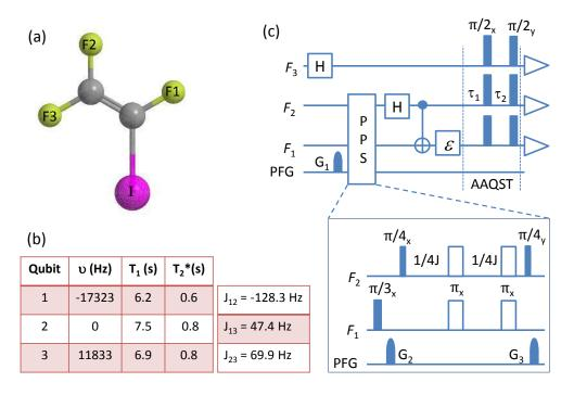
**Figure 3.3:** Molecular structure of iodotrifluoroethylene (a), and the table of Hamiltonian and relaxation parameters (b), NMR pulse-sequence to demonstrate SSPT (c). Pulse sequence for preparing  $|00\rangle$  pseudopure state is shown in the inset of (c).
