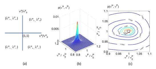
**Figure 5.6:** Characterization of RFI correlations between <sup>1</sup>H and <sup>31</sup>P channels of QXI probe.(a) The  $v^H$  -  $v^P$  plane, (b) the surface plot of the RFI profile  $p(v^H, v^P)$ , and (b) the contour plot of  $p(v^H, v^P)$
