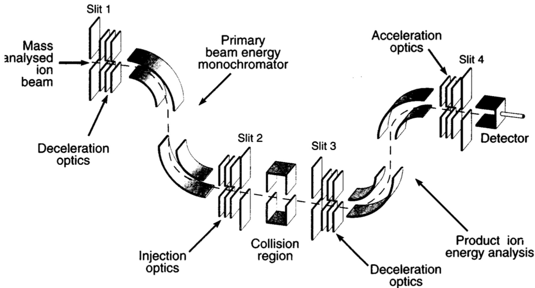
Arrangement of a high resolution energy loss spectrometer
