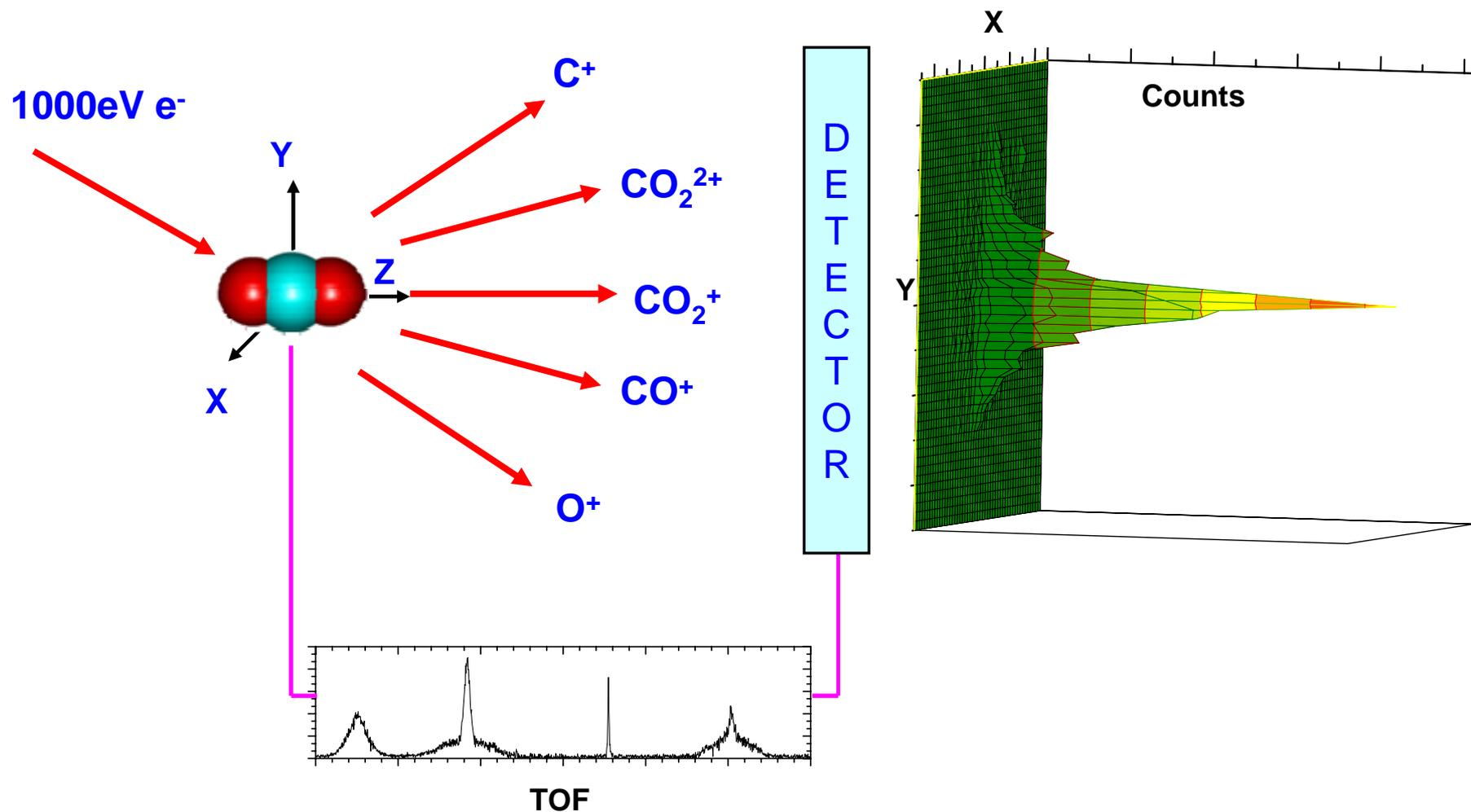
Position and TOF are simultaneously recorded and stored as a list of  $x, y, t$  triplets
