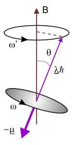
Figure 11: Illustration of the precession (Larmor precession) caused by the torque on the magnetic moment  $\mu$  by a magnetic field  $\underline{B}$ .
