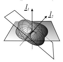
Figure 18: Electron orbitals  $l_1, l_2$  have an overlap depending on their relative orientation and so different vector sums have different electrostatic energy.
