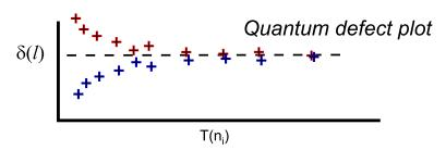
Figure 10: Plot of quantum defect  $\delta(l)$  against Term value, showing effect of choosing  $T_{n_o}$  either too large or too small. The correct value of  $T_{n_o}$  yields a horizontal plot.
