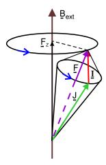
Figure 33: Slow precession of  $\underline{F}$  around  $\underline{B}_{\rm ext}$  whilst  $\underline{I}$ ,  $\underline{J}$  precess rapidly around  $\underline{F}$ .
