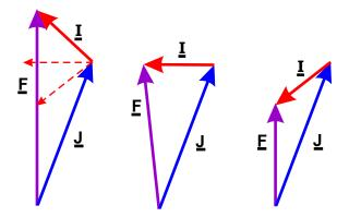
Figure 22: Addition of nuclear spin  $\underline{I}$  and total electronic angular momentum  $\underline{J}$  to give  $\underline{F}$ .
