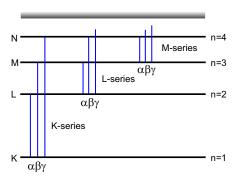
Figure 37: Origin of X-ray series from vacancies created in inner shells.
