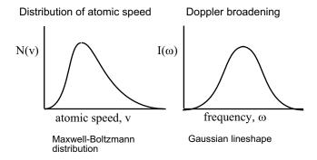
Figure 4: Maxwell-Boltzmann distribution of speeds and the associated Doppler broadening giving a Gaussian lineshape.
