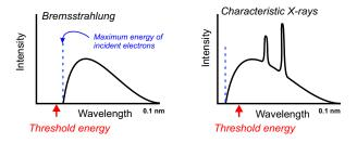
Figure 36: X-ray spectra consist of bremsstrahling and characteristic lines from inner-shell transitions.
