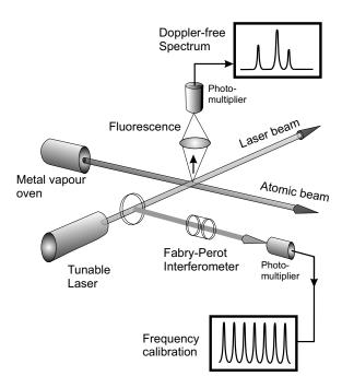
Figure 40: Atomic beam spectroscopy. The light from a tunable laser crosses the atomic beam at right angles and so eliminates the first order Doppler effect. When the frequency of the light is resonant with an atomic transition the resulting absorption is detected by the fluorescence emitted by the atoms.
