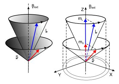
Figure 31: Strong field effect on orbital and spin angular momenta:  $\underline{l}$  and  $\underline{s}$  precess more rapidly around the external field relative to their mutual precession. The projections of  $\underline{l}$  and  $\underline{s}$  on the x-y plane average to zero. As a result only the projections on the z-axis remain to define the energy in the field.
