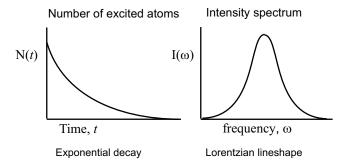
Figure 2: Decay of excited state population N(t) leads to similar exponential decay of radiation amplitude, giving a Lorentzian spectrum.
