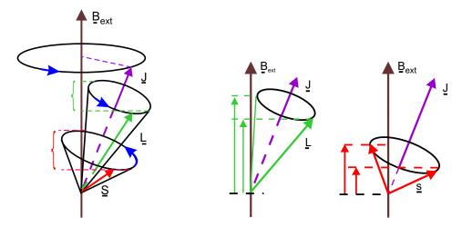
Figure 26: Precession of  $\underline{s}$  and  $\underline{l}$  around mutual resultant  $\underline{J}$  results in projections of  $\underline{L}$  and  $\underline{S}$  on the field axis (z-axis) not being constants of the motion. So  $M_L$  and  $M_S$  are not good quantum numbers.
