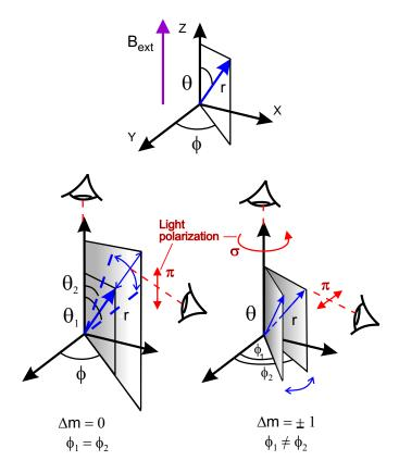
Figure 29: Polarization of Zeeman components viewed along field axis (z-axis) and along a perpendicular axis (x- or y-axis).
