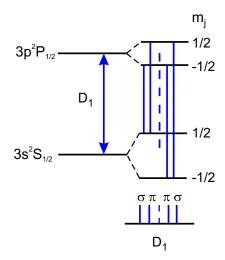
Figure 28: Anomalous Zeeman effect in the  $3\text{s}3\text{p}^2\text{P}_{1/2}$  level of Na. Transitions are governed by selection rules  $\Delta M_J = 0, \pm 1$ .
