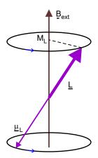
Figure 24: Effect of external magnetic field  $\underline{B}_{\rm ext}$  on an atom with no spin i.e. magnetic dipole due only to orbital motion.
