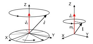
Figure 35: Effect of strong field on hfs: the total electronic angular momentum  $\underline{J}$  precesses rapidly around  $\underline{B}_{\rm ext}$  (z-axis). As a result the nuclear spin  $\underline{I}$  can follow only the time averaged projection of  $\underline{J}$  on the z-axis.
