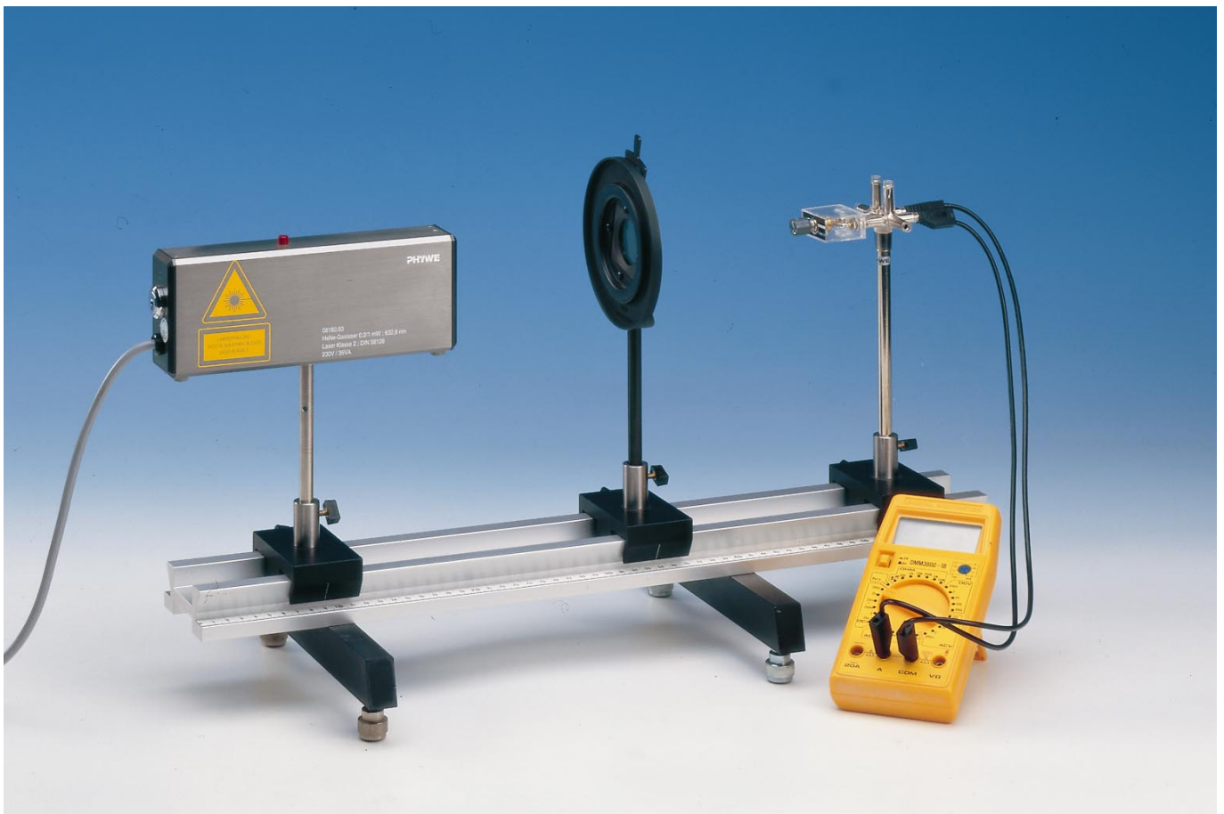
Fig. 1: Experimental set-up: Malus' law.
