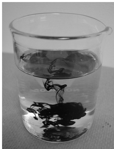
Figure 5.2: Spreading of ink in water.
